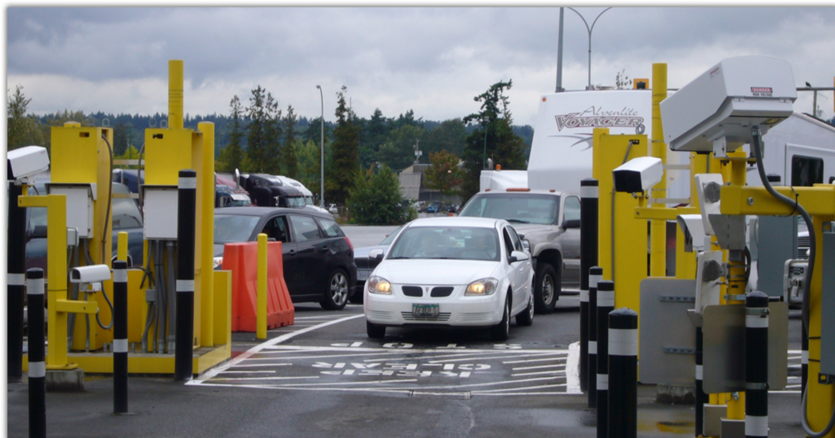
License plate readers (LPR), foreground, at the U.S.-Canada border crossing at Blaine, Wash., help to identify vehicles that may need further scrutiny. Perceptics, LLC, a contractor for Unisys Corp., is installing this advanced technology and other technological upgrades for the U.S. Department of Homeland Security at the U.S. borders with Canada and Mexico between now and mid-2009 under the Western Hemisphere Travel Initiative.
