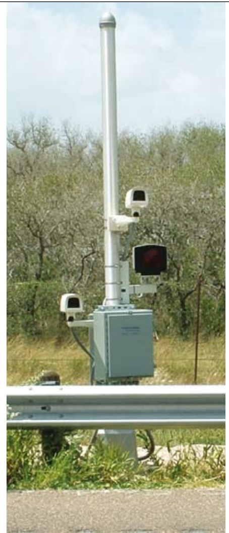
📌 Electronics are in a weatherproof enclosure
