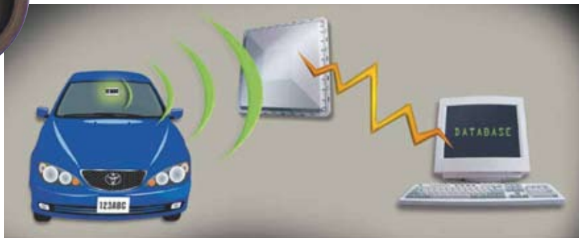
⬆ EVR uses RFID to identify vehicles and validate the identity, status, and authenticity of data
