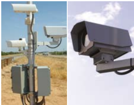
⬆ The Perceptics system automatically captures, identifies and records the alphanumeric code, state/province of origin, and country of origin
