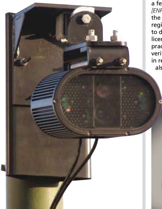
⬆ PIPS's P382 Spike2 is ideal when multiple lane coverage is required from a single ALPR unit
